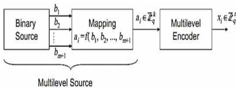
**Figure 1: Non-Binary BCM Encoder Structure**
